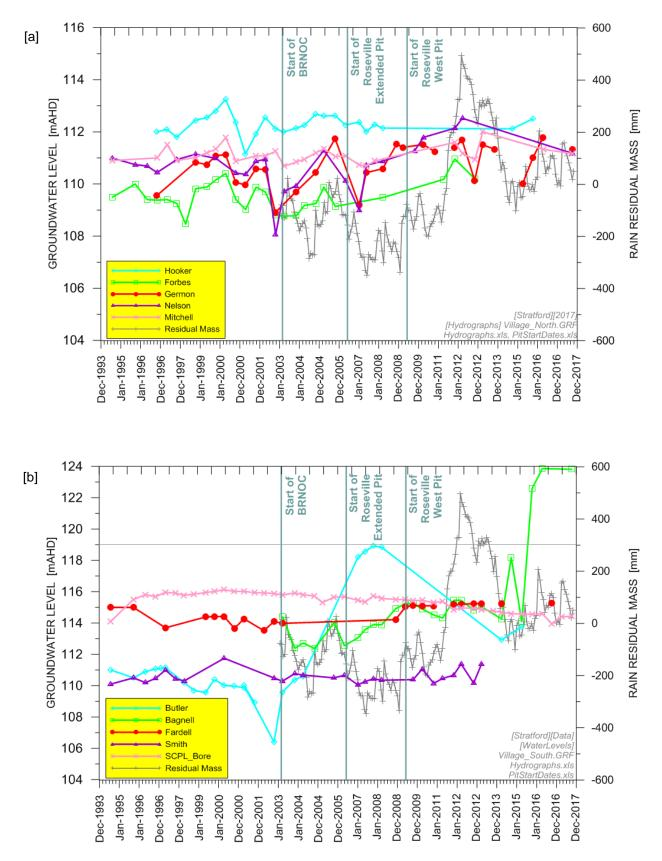
Figure A4. Groundwater hydrographs at Stratford Village: [a] north; [b] south
