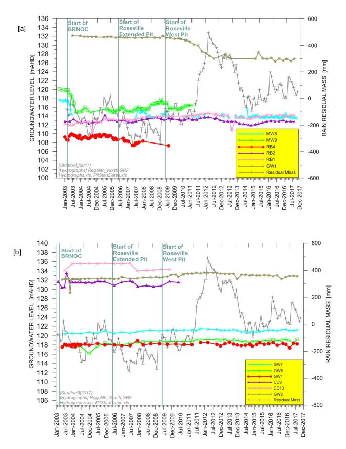
Figure A2. Groundwater hydrographs in regolith: [a] north; [b] south
