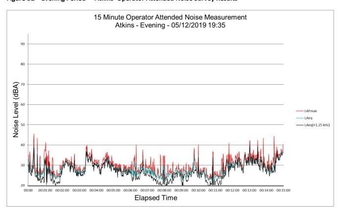
15 Minute Operator Attended Noise Measurement Atkins - Night - 06/12/2019 00:37 90 80 Noise Level (dBA) LAFmax – LAeq(<1.25 kHz)
