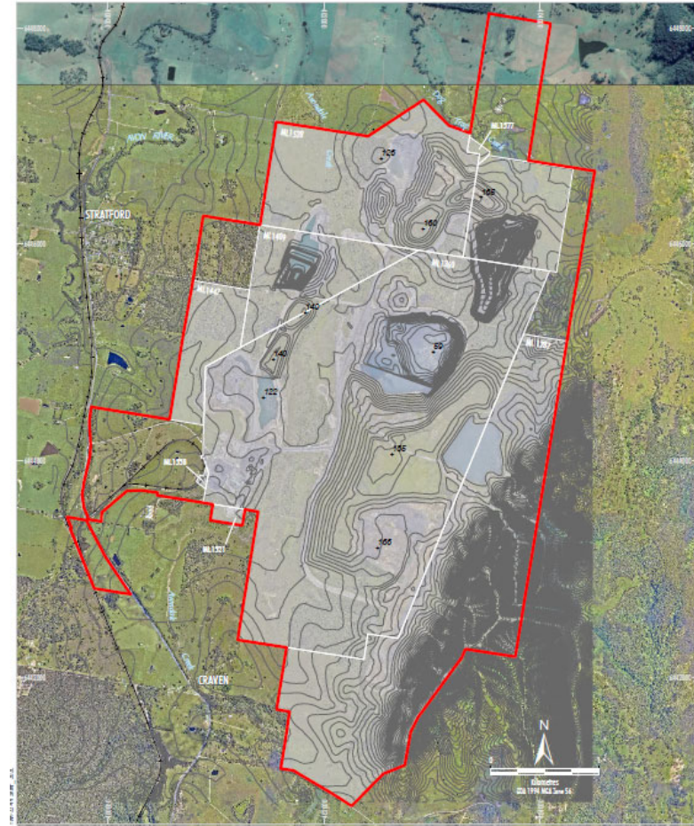
Source: Orthophoto - Yencord (2021); LPI (2016); NSW Department of Planning & Environment (2017) LEGEND Project Approval Boundary Coal - Current Titles Final Landform Contours (5 m Interval) STRATFORDCOAL Part of the Yancoal Australia Group STRATFORD EXTENSION PROJECT Final Landform Contours
