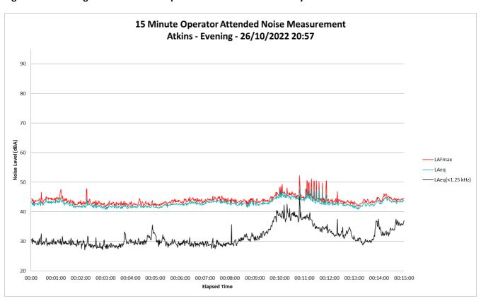
Figure B3 – Night Period – 'Atkins' Operator Attended Noise Survey Results
