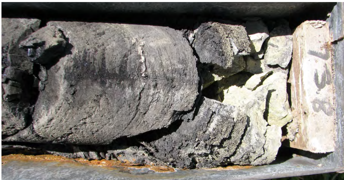
Plate 3: Pyritic zone (approx. 0.5 m thick) in carbonaceous claystone and coal (Triple Seam) with jarosite and sulphate salts due to partial oxidation of pyrite. Hole SC48 at 73.9 m.
